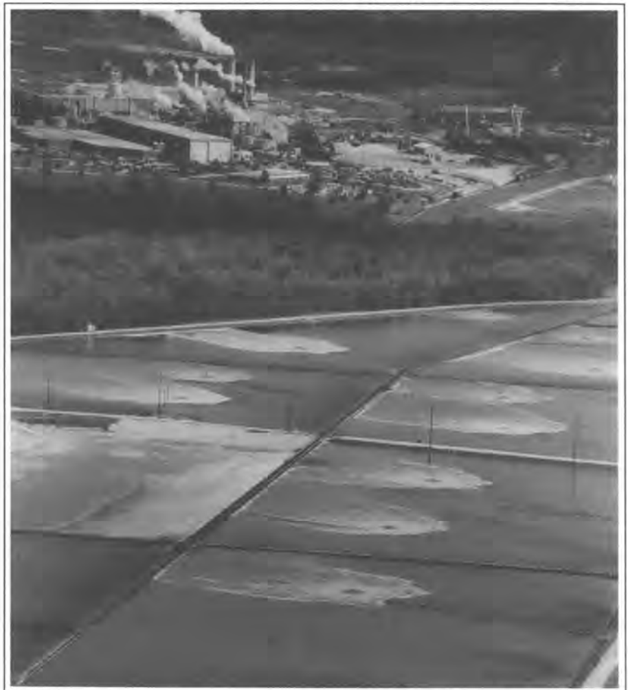
SINKHOLES HAVE OPENED IN SOME OF THE PONDS THAT PROCTER & GAMBLE USES TO TREAT WASTE FROM ITS CELLULOSE MILL IN PERRY, FLORIDA.
